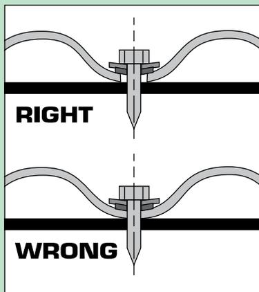
Allow for proper expansion in all drilled holes. A diameter of 5/64" larger than fastener is recommended.
